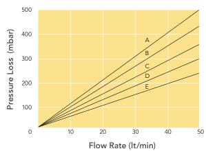
A=0.1μm B=0.2μm C=0.45μm\* D=1μm\* E=00P\* \*G Grade Only
