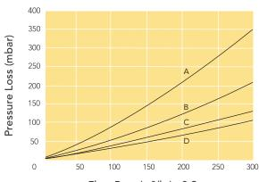
Flow Rate (m³/hr) - 0.2µm A=0 Bar B=1 Bar C=2 Bar D=3 Bar
